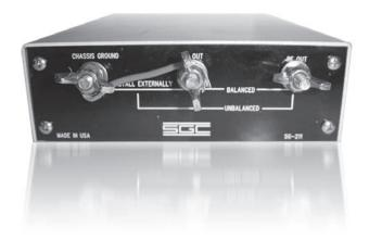
A wide variety of antennas can be connected to the SG-211. A set of wing nuts for connecting balanced or unbalanced antennas is provided on the back.
