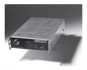
The SG-211 is in an Aluminum Irridited case. RF comes in through an SO-239 connector on the front of the case and goes out through balanced and unbalanced connectors on the back. Internal construction is normal for portable or fixed location use. Corrosion resistant hardware and passive alloys are used throughout.
